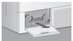
• Unlock the air cooler by turning the blue locking levers inwards.
