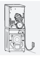
Washer-dryer tower When using the same siphon for the washing machine and the dryer, it might become necessary to install a check valve on the back wall of the dryer.
