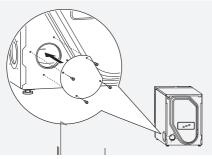
Close the exhaust opening at the back of the dryer with the cap removed earlier.
