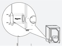
Remove the cover of the desired exhaust opening.
