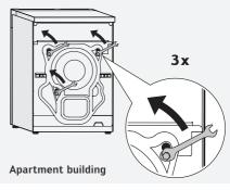
Loosen hexagonal screws with a spanner (spanner size 13), until the screws can be moved freely.
