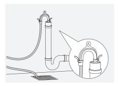
Fasten the hose on both sides with a cable tie.
