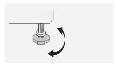
If necessary, adjust the height of the feet of the machine by turning them.
