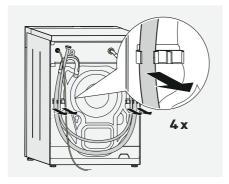
Remove the hoses and cables from their holding straps.
