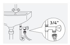
Carefully turn on the water tap to make sure that the connections are not leaking.
